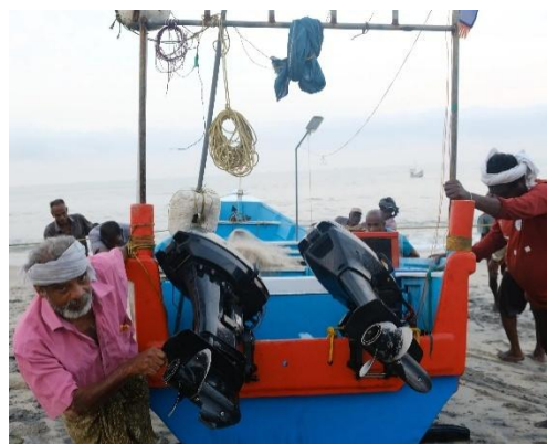
Hybrid propulsion system installed on a fishing vessel to enhance fuel efficiency and reduce carbon emissions.
