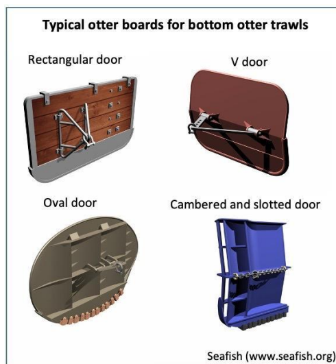
Different otter board designs illustrating hydrodynamic features for improved trawl efficiency.
