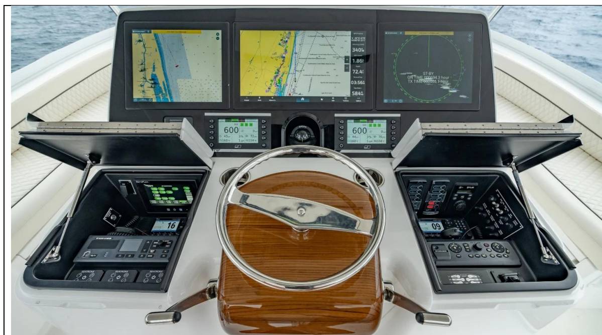
Figure 1. Modern fishing vessel equipped with advanced navigation and fish detection technologies such as GPS, radar, sonar, and electronic chart systems.
